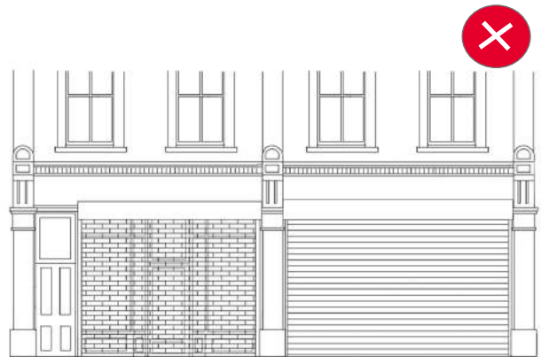
Picture 23. External Roller shutters are not appropriate.
